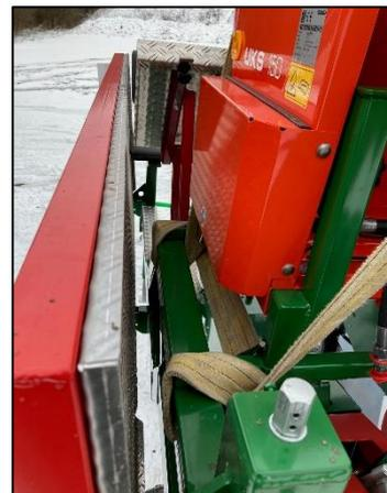
*Lifting with slings around the side frame*
