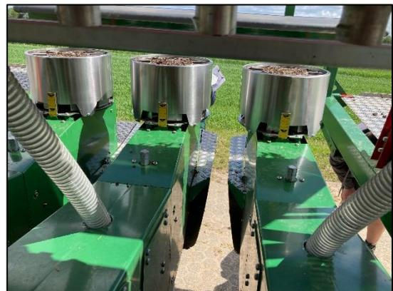
*Scales for setting depths on the gauge wheel, feeler wheel and planting coulter*
