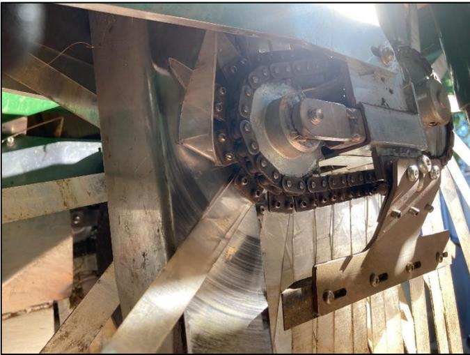
*Blockage due to stuck slat*
