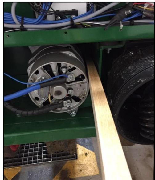
*Tensioning the alternator V-belt*
