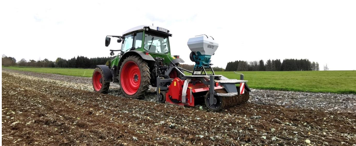
Figure 31 MulchTec-RotoSeeder used to sow a winter cover crop with minimal soil disturbance after mowing cabbage residues. Image: Johannes Storch (2023)
