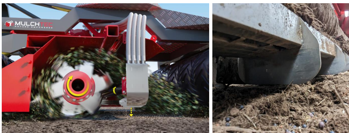
Figure 30 Functionality of MulchTec-RotoSeeder (left) and seeder bar with cover crop seed (right). Illustration: MulchTec, Germany (2023) and Johannes Storch (2023)
